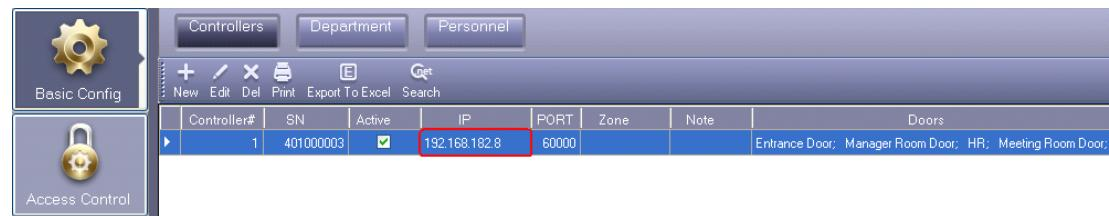
The controllers are separated into different network . Each controller must be assigned a unique IP address .
